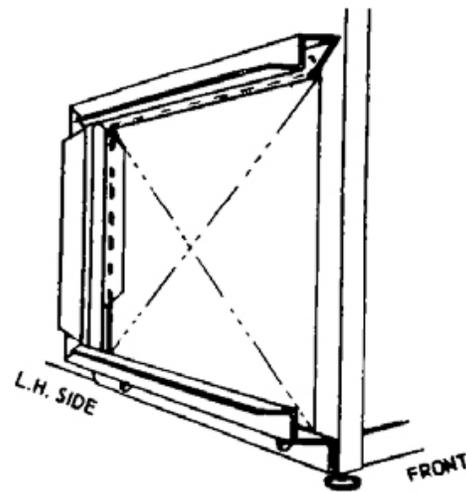
The required disposable panel filter size is 16 X 25 X 1-in. There is no filter supplied with this accessory. The installing contractor must provide and install the recommended filter.
