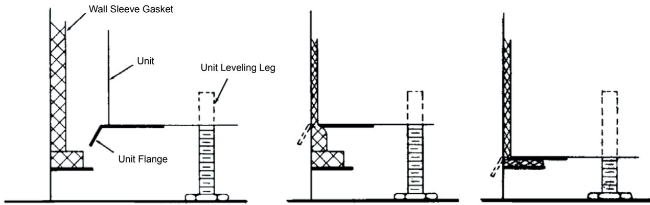
1. Raise unit by means of leveling legs unit Flange must clear bottom angle of wall sleeve.
